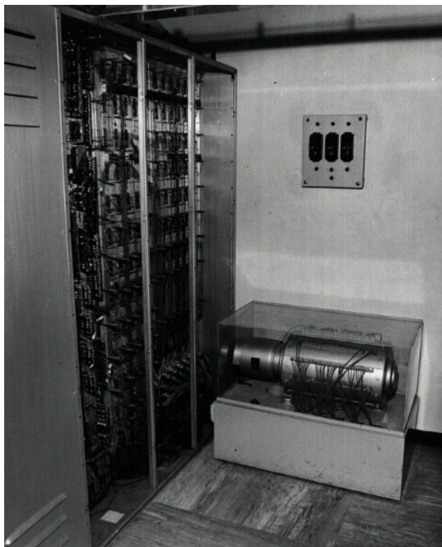
Figure 5: The magnetic drum memory of the CEP, 1961. It has a capacity of 16384 36-bit words. (credit: www.cep.cnr.it).
