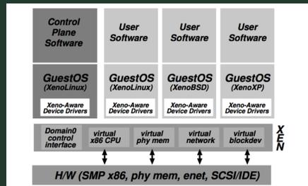
Figure 1: The structure of a machine running the Xen hypervisor, hosting a number of different guest operating systems, including Domain0 running control software in a XenoLinux environment.
